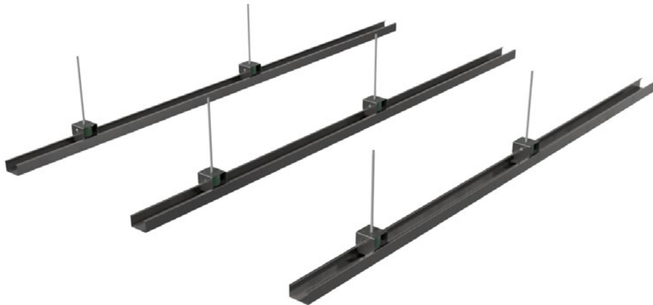
Figure 1: The VT-SFC system contains only primary profiles. Tested with 25 mm elastic pads. In the tests the hangers were mounted with c/c 900 mm and the profiles were mounted with c/c 450 mm.
